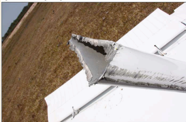
Figure 5 – Severed right wing strut
