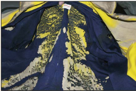
Figure 6a—Much of the polypropylene undershirt (blue) melted during the full-scale flame engulfment test.
