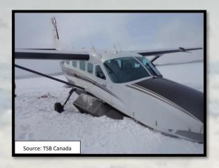
At approximately 1414, the pilot made the decision to initiate a go-around; however, as power was being applied, the aircraft collided with the frozen surface of Family Lake, 0.75 nm from the threshold of Runway 36 (Figure 1). The aircraft remained upright and slid to a stop on the snow. The pilot and 6 passengers received minor injuries and were able to egress from the aircraft. They were rescued by passersby on the nearby ice road. The aircraft was substantially damaged.
