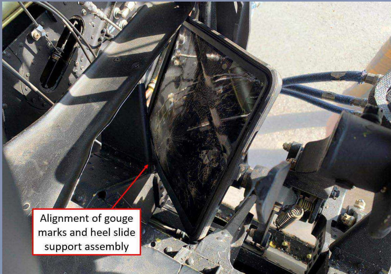
Figure 4. The iPad impinged in between the co-pilot's left pedal and the airframe. The lower left corner of the iPad is lodged into a small corner of the airframe. The gouges in the iPad aligned with a sharp, vertical metal piece of the heel slide support assembly.
